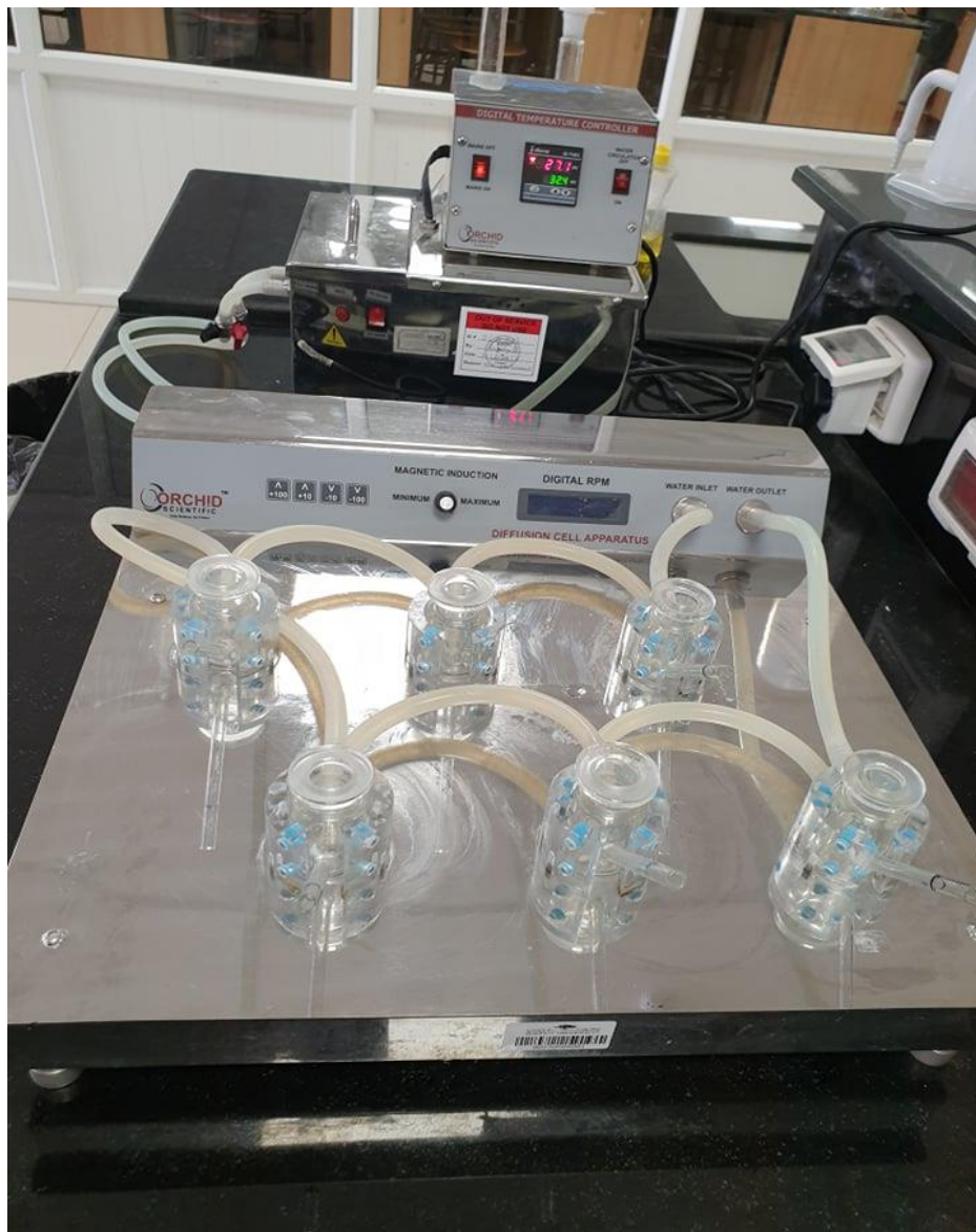
Figure 3. 1: Franz Diffusion Cell used in the study of diclofenac Sodium skin permeation.
